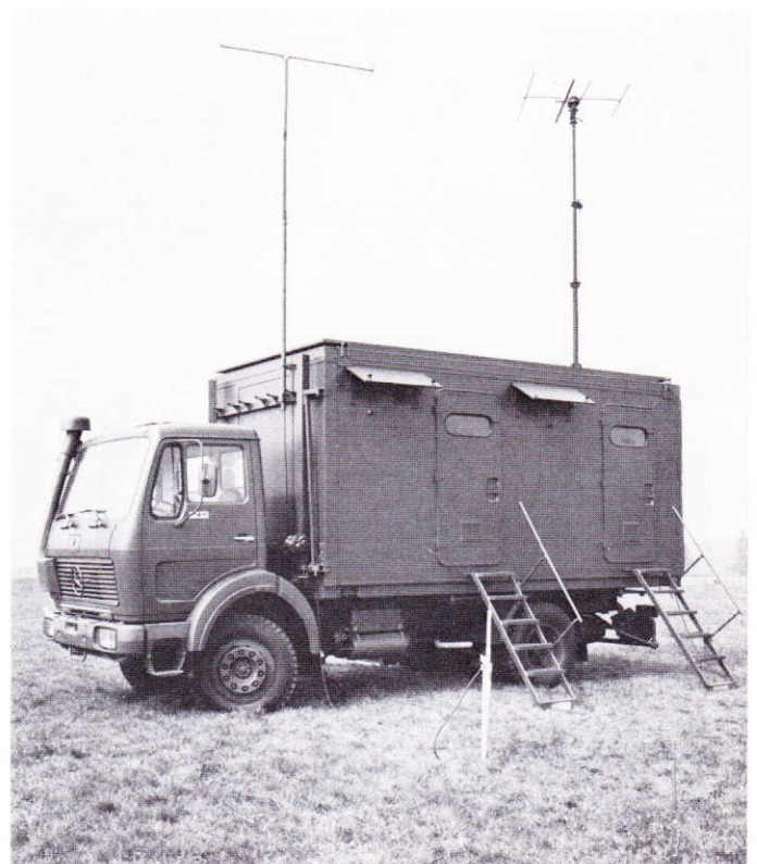
Mobile Rundfunksendestation Mobile broadcasting transmitting station
