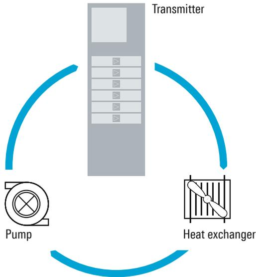
Liquid cooling has been used for terrestrial TV transmitter systems for several years. The closed cooling circuit encompasses the transmitter, a pump unit and a heat exchanger.
