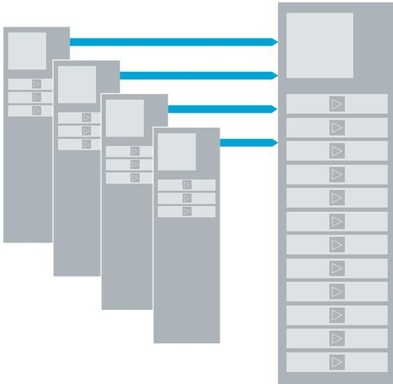
The MultiTX system concept from Rohde&Schwarz allows up to four transmitters to be installed in a single rack – now also for liquid-cooled FM high-power transmitter systems. This saves a considerable amount of space.
