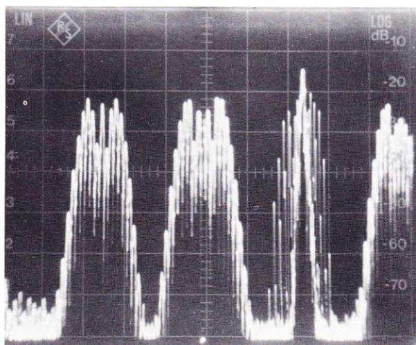
Fig. 3 IF analysis (log display); modulation spectrum of one occupied and three vacant public land-mobile radio channels; sweep width 200 kHz, resolution 1.5 kHz
