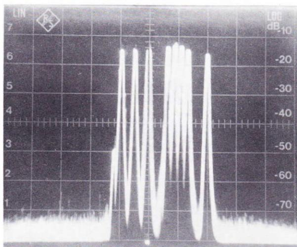
Fig. 2 IF analysis (log display); sweep width 2 MHz, resolution 15 kHz; the marker identifies the public land-mobile radio channel picked up by the receiver
