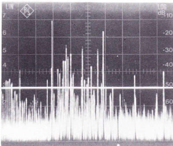
Fig. 5 Expanded-extract display of momentary band occupancy (start/stop) with superimposed receiver tuning marker and recorder response level line
