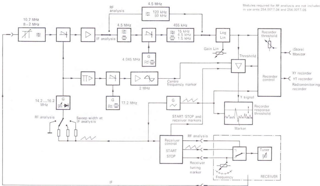
Fig. 6 Block diagram of Panoramic Adapter EZP
