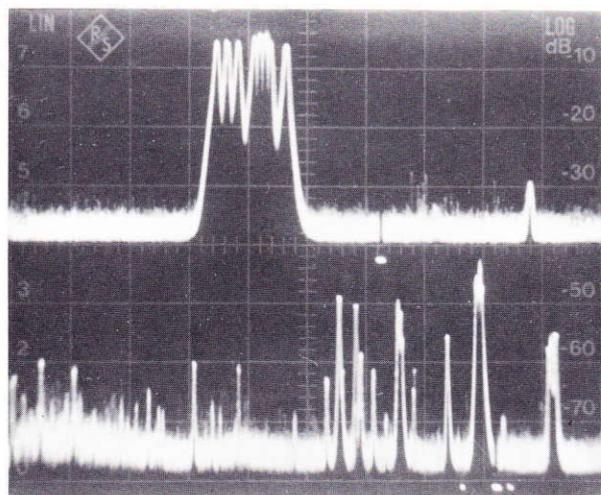
Fig. 1 RF analysis (log display); range display (from 105 to 172 MHz) with 120-kHz resolution (lower line); start/stop and receiver tuning markers define the section displayed on the upper line with 50-kHz resolution (public land-mobile radio channels)
